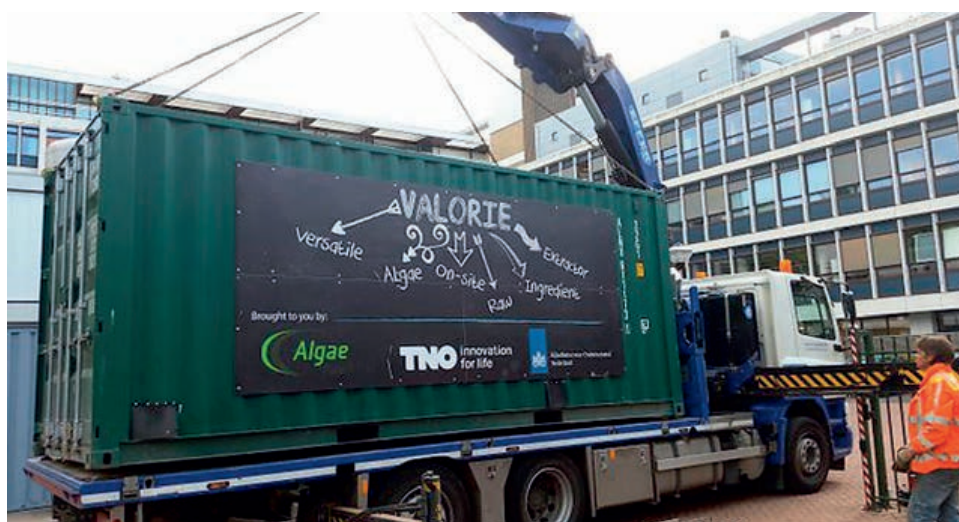
The unit operations have been mounted in a 20-foot container to allow on-site trials, next to where the algae are produced since processing of fresh algal biomass is highly desired
